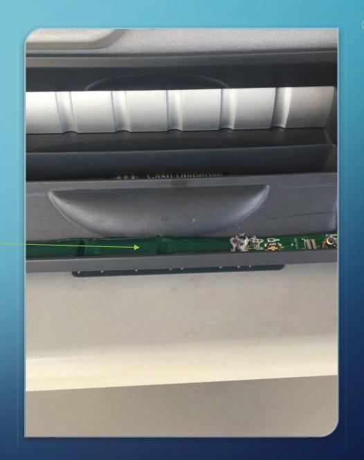
This is the skimming device removed from the ATM cash dispenser frame. Notice the small hole in the corner of the frame. This is unusual. The small hole provides a view for the camera lens.
