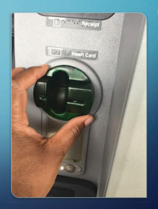
This skimming device removed from the ATM card reader looks identical when compared with the actual reader.
