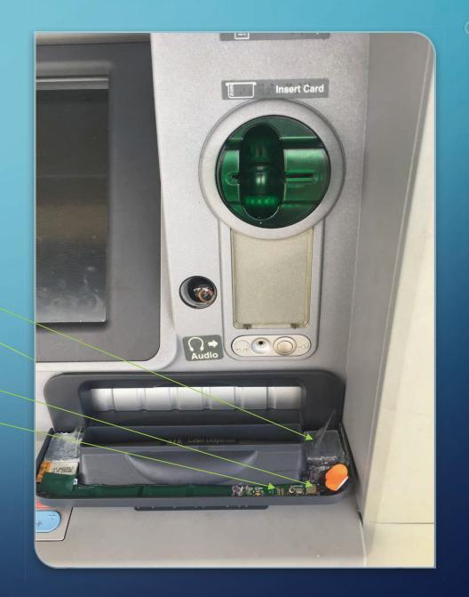
This is the skimming device removed from the ATM cash dispenser. The frame is attached with adhesive and is placed directly over the existing ATM cash dispenser frame.
