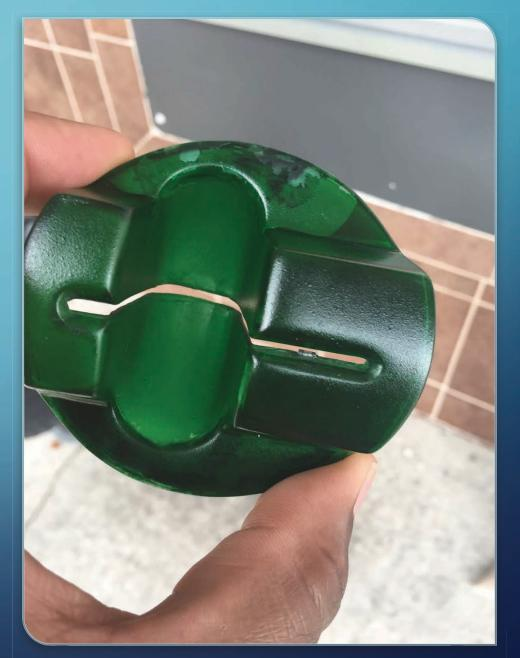
This is the same skimming device removed from the ATM card reader. But when you remove the skimming device and flip it over, you can see the white adhesive tape and the skimming hardware used to capture information from the magnetic strip. This particular device has a female connector for transferring card information and onto another device which can be used to create new cards.
